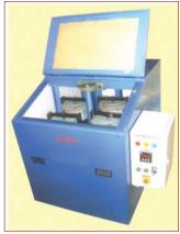
rotate in a direction opposite to that of the rotating turret. This particular model is available in 12 litres capacity. Technical Specifications – Overall capacity: 12 litres (0.40 cu.ft); Width: 750 mm (29.5 inch); Depth: 1000 mm (39.4 inch); Height: 900 mm (35.4); Motor: 1.5 HP; RPM: 180 mm. Ceramed Engineer's products range includes: Centrifugal High Energy Machines, Centrifugal High Energy Polishing Machines, Rotary Driers, Spiral Type Vibrators, Tub Vibrators, Vibratory Driers, etc.
