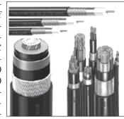
nded circular/compacted/sector shaped. Insulation is PVC; Mechanical protection: Galvanized steel wire/strips/double helical steel tape; aluminium wire amounting for single core cable; Inner and outer sheath – PVC black/grey or as per requirement.
