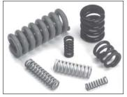
of Chrome Silicon or Music Wire material. Available in various sizes to fit most standard diameters and in five color-coded durable load ratings. HEFTY<sup>TM</sup> Die Springs are shot-peened to extend life, preset to prevent length loss in operation, and powder coated to prevent corrosion. This series is ground with closed ends to provide appropriate squareness and an adequate large bearing end surface. Contact:
