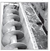
dling highly abrasive material can be designed without hanger bearings up to the length of 12 m. MASYC an ISO 9001: 2000 Company has a formidable presence in the market in Bulk Material Handling Systems and Equipments, and has more than 30 years of experience in turnkey execution of Bulk Material Handling Systems. Its products range suit all the requirements in different processing industries like Cement, Steel, Coal, Pulp and Paper, Glass, etc.
