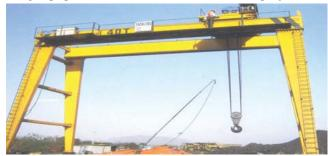
maintenance Factories, Power Stations, Large Water Works, Railway Yards, Harbours, Warehouses, Construction Sites, Transporters, Mines, Quarries, Heavy Fabrication Units, Contracting Firms, etc. It finds numerous applications such as loading and unloading trucks, heavy pipe laying in trenches, erection of bulky equipment, shifting of heavy load, etc. The Crane capacity is from 1 ton to 80 tons.
