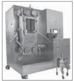
feeding and discharge. Gentle fluidization as a result of small depth of material. Integrated WIP system with access ports for easy cleaning and maintenance. Can be used for a process range between 1 kg and 15 kg. Contact:
